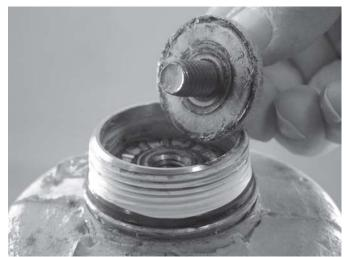
Thrust Washer and Bearing
