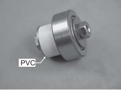
Roller Half of Bearing with insert tool
