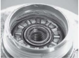
Greased Thrust Half of Bearing
